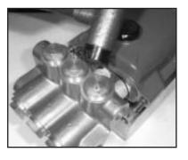
firmly into the retainer with a wooden dowel making certain that the spring side of the seal is installed first and that the seal sits squarely in the retainer.
